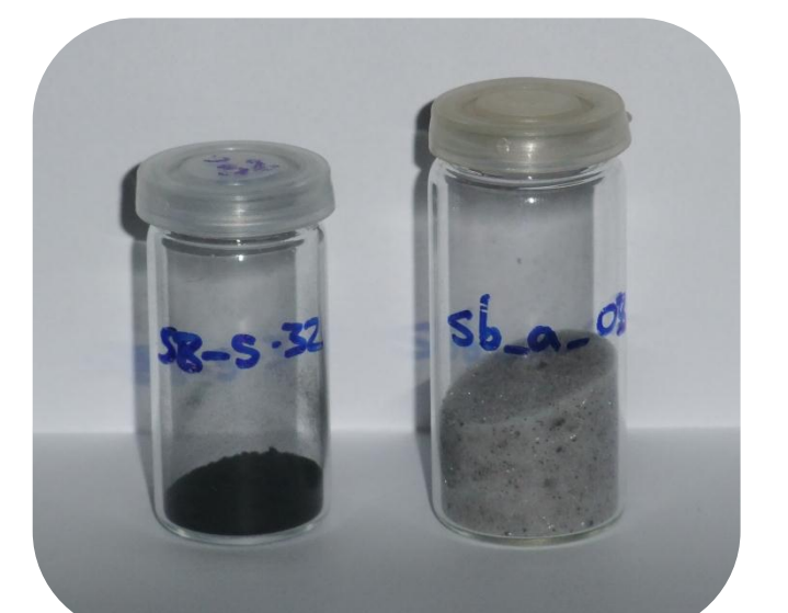
Fresh catalyst coated with Li/K/Cs[OAc] Catalyst with inert material after reaction
